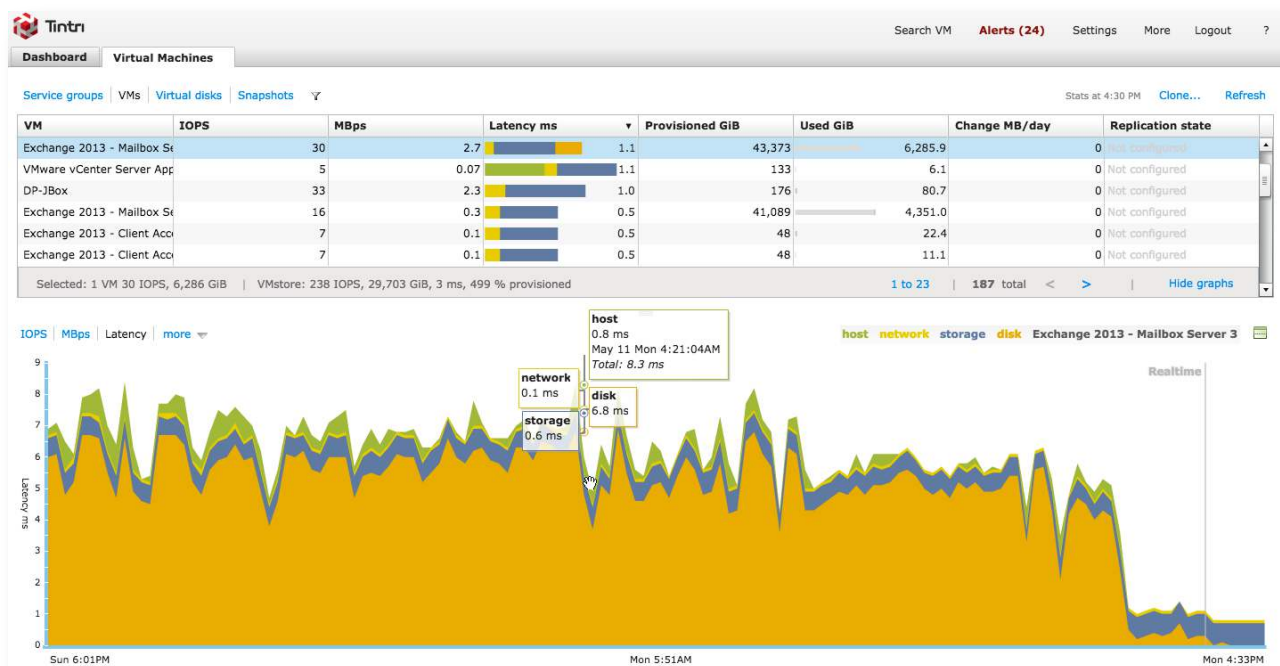
Figure 2 – Tintri VMstore dashboard showing per-VM statistics and latency measurements
