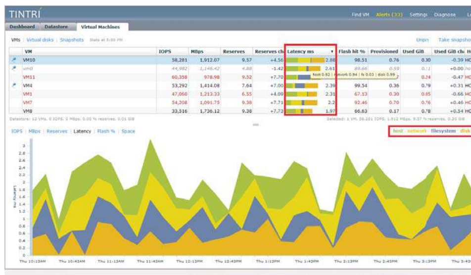
Figure 1: Tintri VMstore displays end-to-end latency statistics for each VM for automated bottleneck visualization.
