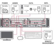
Plug in power cables and stand back - the system will begin the boot process.
