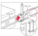
Insert your EC6000 into the outer rails, install the two longer screws to keep it in place, one on each side, then attach the bezel. Stand back and admire your handiwork.
