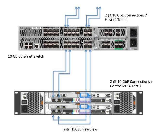
**Figure 2: Physical System Connectivity**
