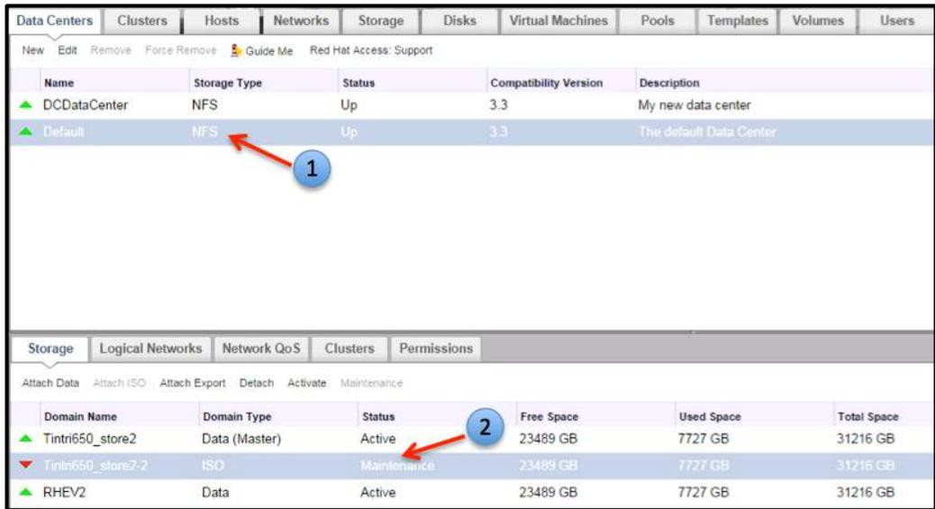
Figure 12: Detach RHEV Storage from a RHEV Data Center.
