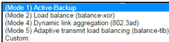
Figure 7: RHEV supported Network Bonds.
