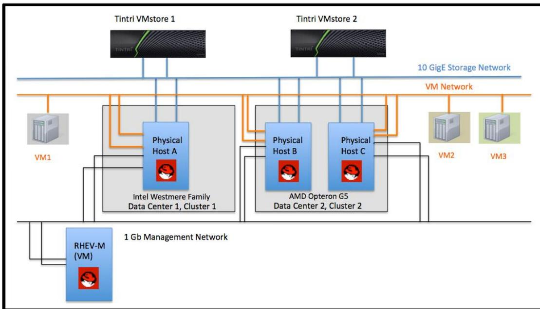
Figure 1: Architectural overview of Tintri VMstore deployment in a RHEV Environment.
