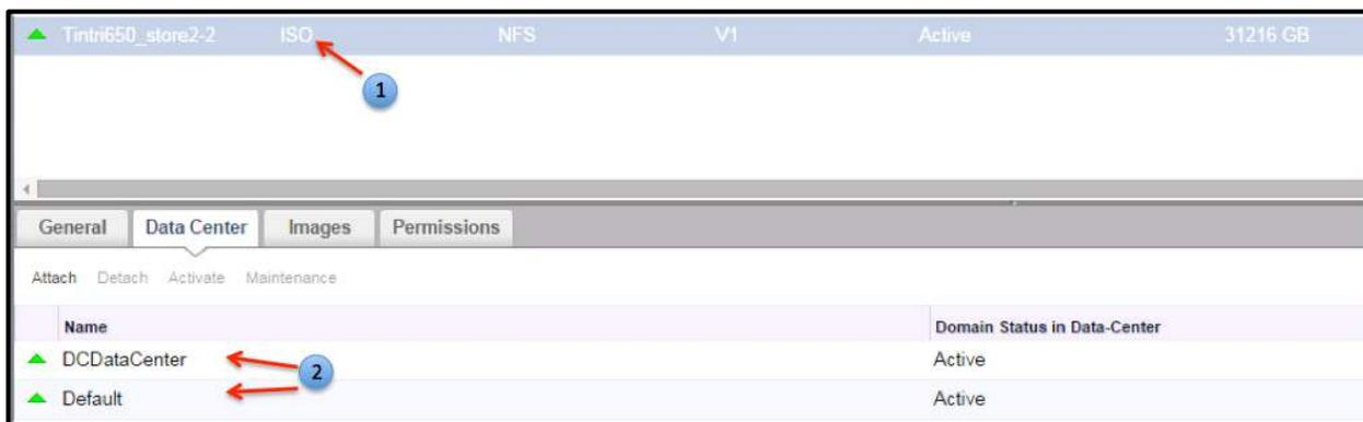
Figure 11: Tintri NFS submount shared between 2 RHEV Data Centers as an ISO Domain.
