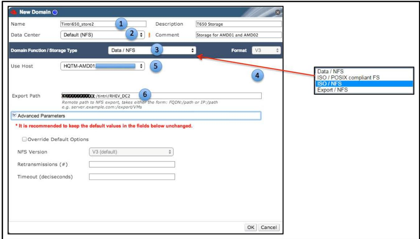
Figure 9: Adding a new Storage Domain to a RHEV Data Center.
