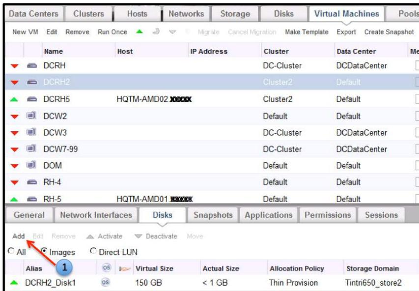
Figure 19: Adding Virtual Disk to an existing Virtual Machine.
