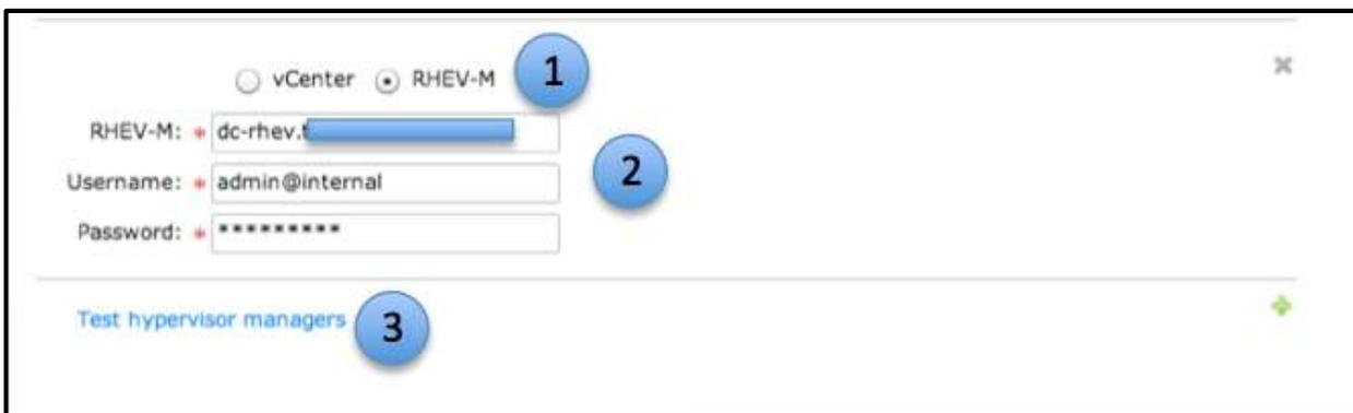
Figure 5: Configuring RHEV-M with Tintri VMstore.
