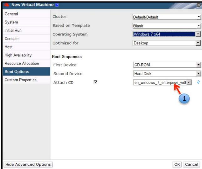
Figure 16: Attach CD to Virtual Machine.
