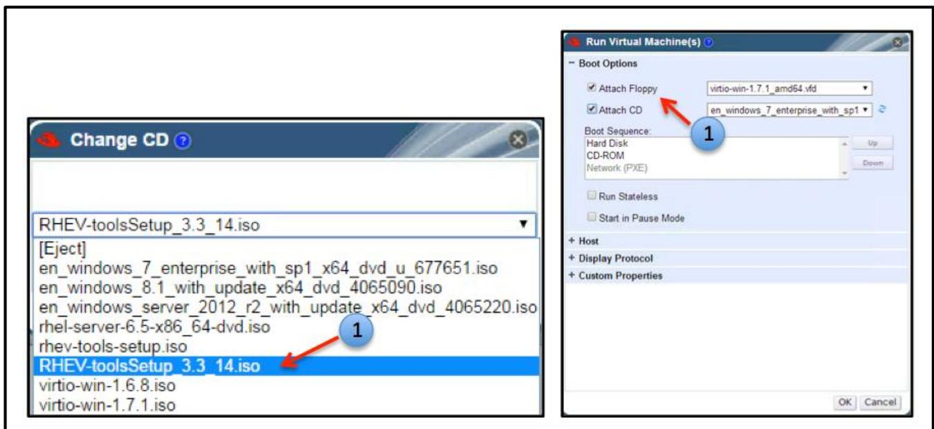
Figure 20: Using Change CD or Attach Floppy to install RHEV Virtual Machine drivers.
