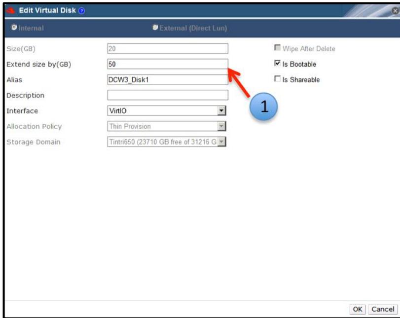
Figure 18: Extend existing Virtual Disk size.
