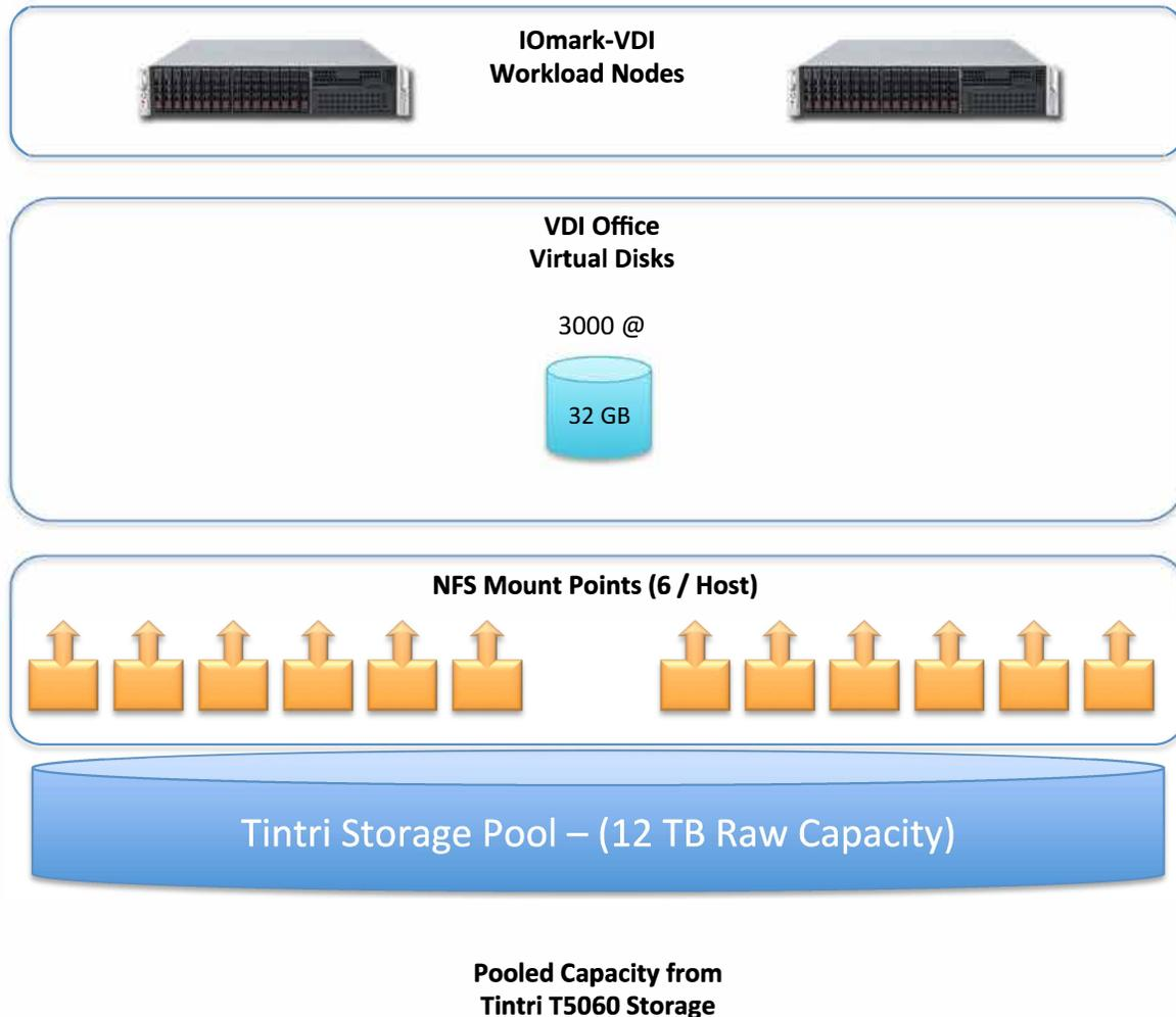
**Figure 1: Logical System Configuration**
